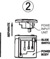
Detach power input unit to reveal fuse socket, shown in figure 3.
