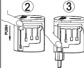
Depress slide-switch and slide down fully as shown to reveal pins. Release the slide-switch to lock the pins in place.
