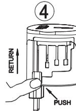
To retract the pins after use, depress the slide-switch and slide upward fully as shown. Release the slide-switch to lock.
