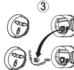
To replace the fuse, use a screw-driver to release the cap. Use only the correct type of fuse. (Fuse specifications on last page)
