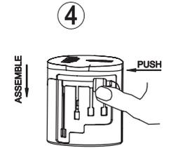
To re-assemble, place fuse cap back and screw to close. Then re-attach the power input unit. Push slide-switch left.
